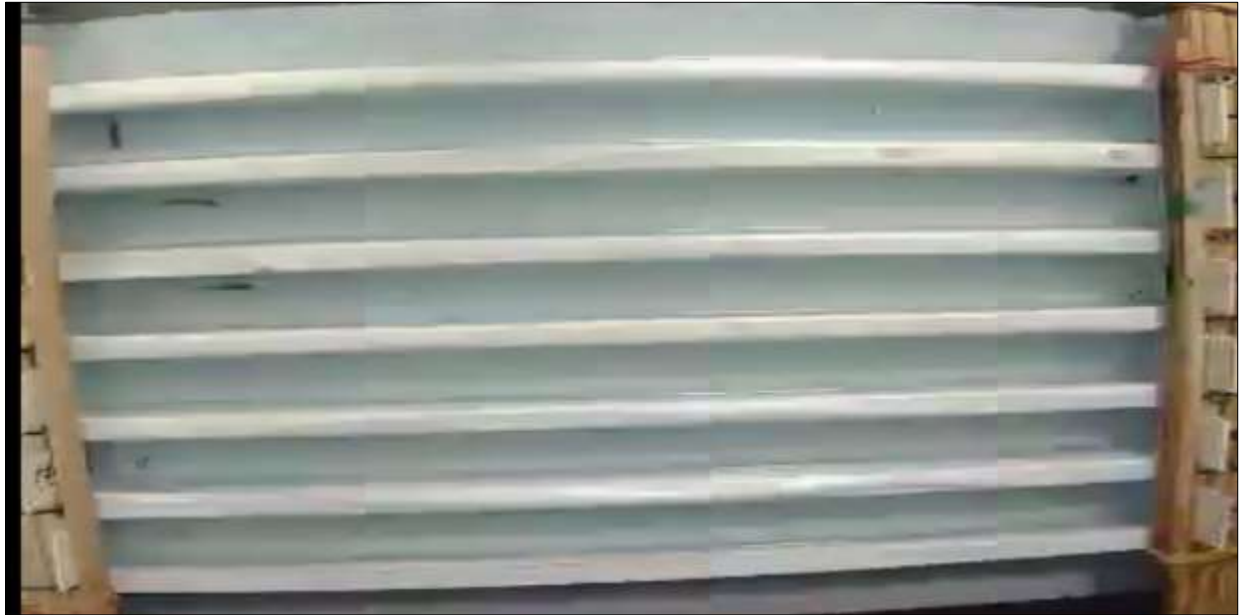
Figure 2 Swimming tunnel designed for six individual fish to compete in performance against water current
