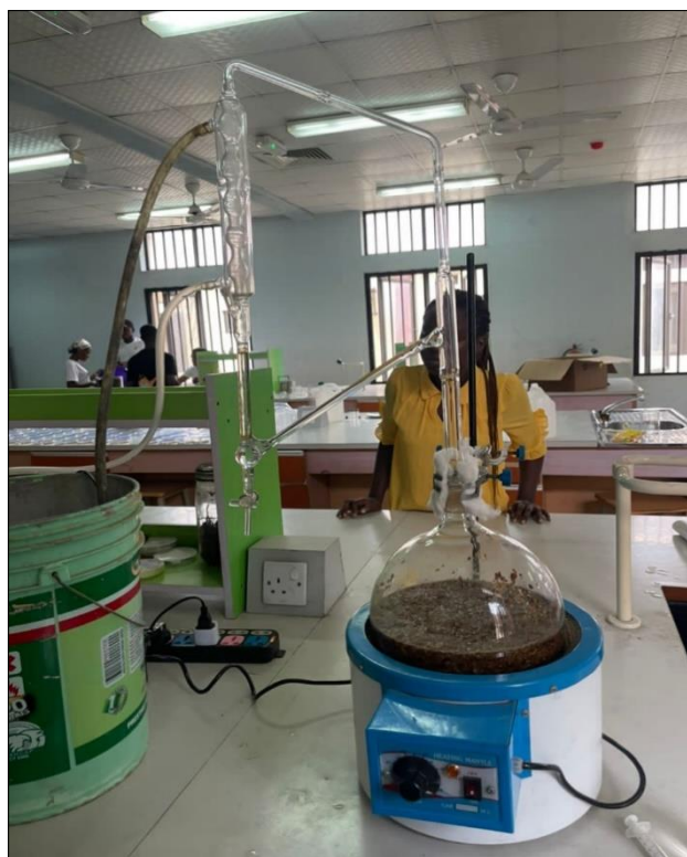
Figure 1 Extraction of the Essential Oil using Hydro distillation Method
