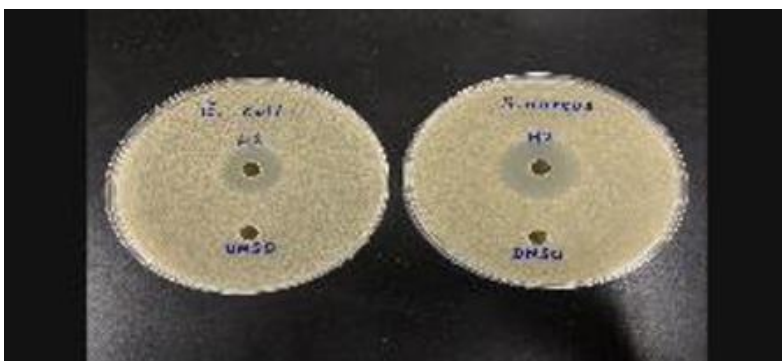
Figure 16 Representative agar well diffusion plates for compound H2 against E. coli and S. aureus , with DMSO as the negative control.
